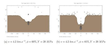
Figure: Comparison of crater profiles on highly porous surfaces (60 % and 85 %).
