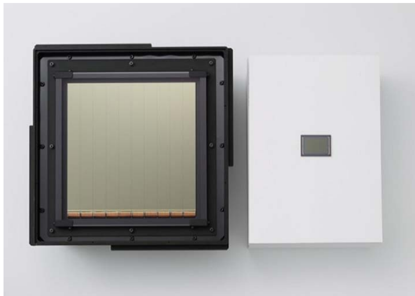
Figure: A new large-format CMOS sensor (left) and a 35-mm full-frame CMOS sensor often used in digital single-lens reflex camera product (right). Image was provided by Canon Inc.
