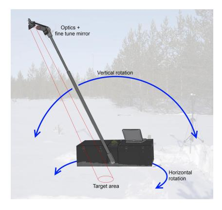
**Figure:** FIGIFIGO consists of the following main components: casing, measurement arm, rugged computer, and a sunphotometer on a tripod. The casing contains the main sensor ASD FieldSpec Pro FR optical fiber spectroradiometer (350–2500 nm), most of the electronics, and batteries. The active optics system is located horizontally at the top of the measuring arm, and is looking down to the target through a mirror.
