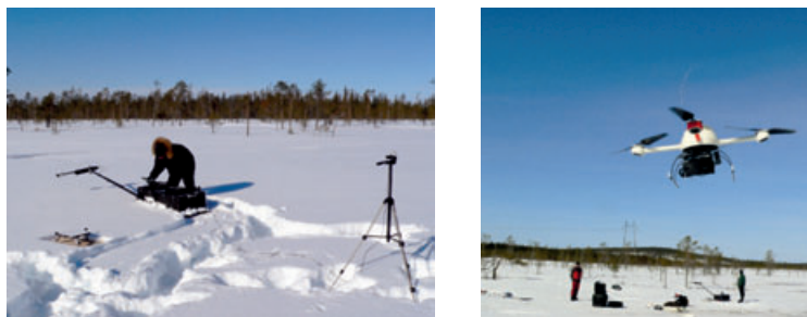
Figure 2. Left: FIGIFIGO measuring snow, foreground left the Spectralon reference panel, right the sky monitoring pyranometer. Right: Microdrone md4-200.
