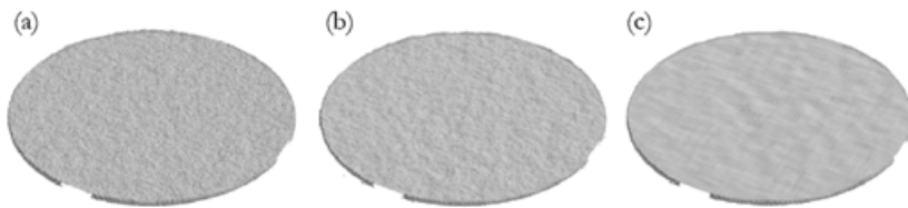
Figure 1. Three realizations of the surface model. All the surfaces have \tau = 500 nm and \sigma = 20 nm. The leftmost surface has \kappa = 1/2 (exponential correlation), the middle \kappa = 1 , and the rightmost has \kappa \rightarrow \infty (Gaussian correlation).
