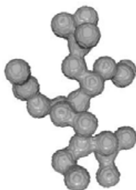
Figure 2. DDSCAT shape data of sintered aggregate of Fig. 1b.
