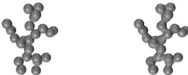
Figure 1. a) Shape of DLA aggregate, r = 25 nm, D_f = 1.8 , N = 24 . b) Shape of sintered aggregate with sinter parameter A/A_0 = 0.86 .
